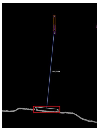
Cordel AI-Classification of 3D Point Cloud (left) and extracted 2D OLE Height and Stagger Cross-Section (right)
